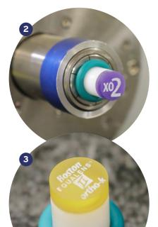
An alternate method of lathing the base curve is to block the button onto a flattopped arbor (2). This approach ensures there is no excessive collet pressure exerted on the button material.
